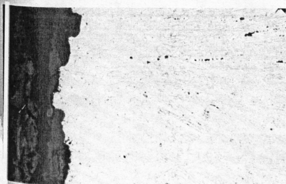
Plate 23 Microstructure illustrating the decarburized zone of an annealed white iron casting. The interior showing graphite nodules is the malleabilized cast iron product.
